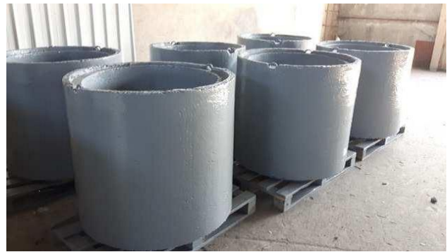
Fig. 2 Tested concrete rings covered by polyurea coating system
