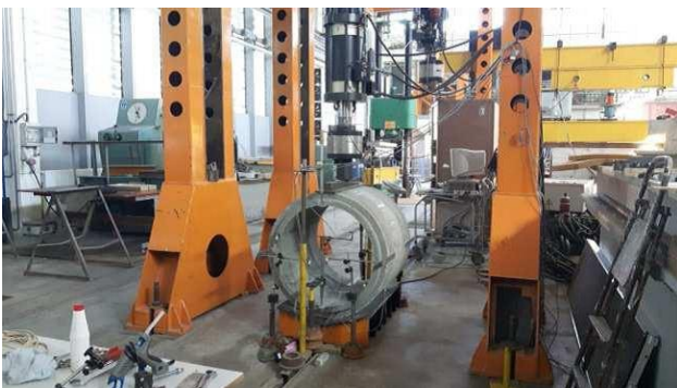
Fig. 6 Frame used in testing concrete rings
