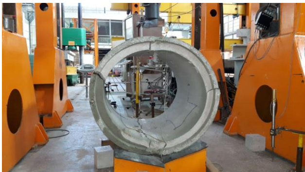
Fig. 8 Concrete ring with polyurea coating on external surface after destruction and unloading
